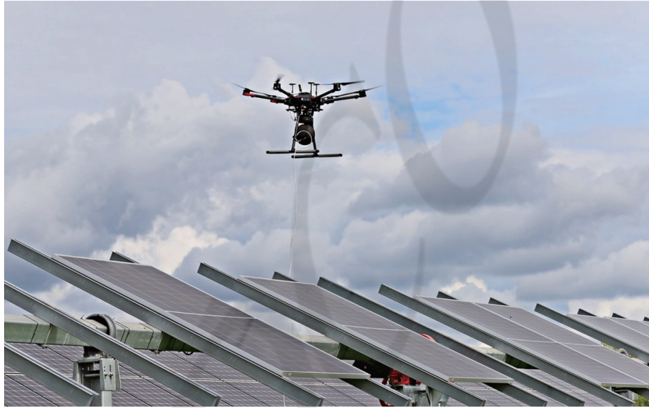
UAV-based electroluminescence imaging technology
